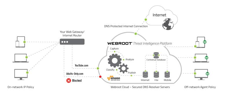
How Webroot SecureAnywhere® DNS Protection works
